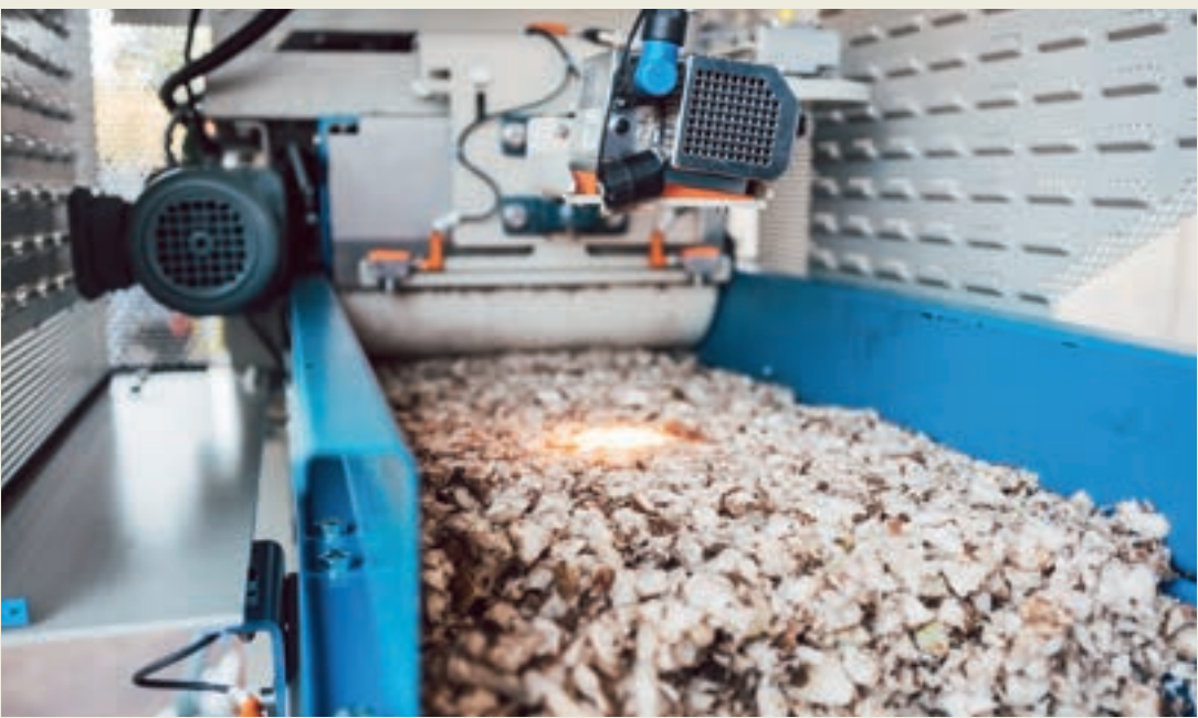
In-flow NIRS measurement includes the whole heterogeneity of beets and replaces mixing
