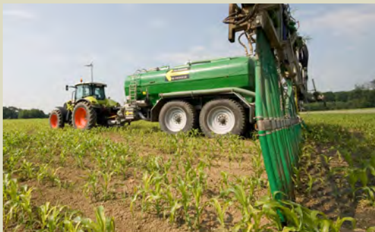
Liquid digestate application at the 4-leaf stage (V4) via a drop leg system
