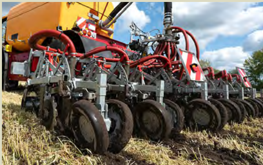
Liquid digestate application pre-drilling via a strip-till system
