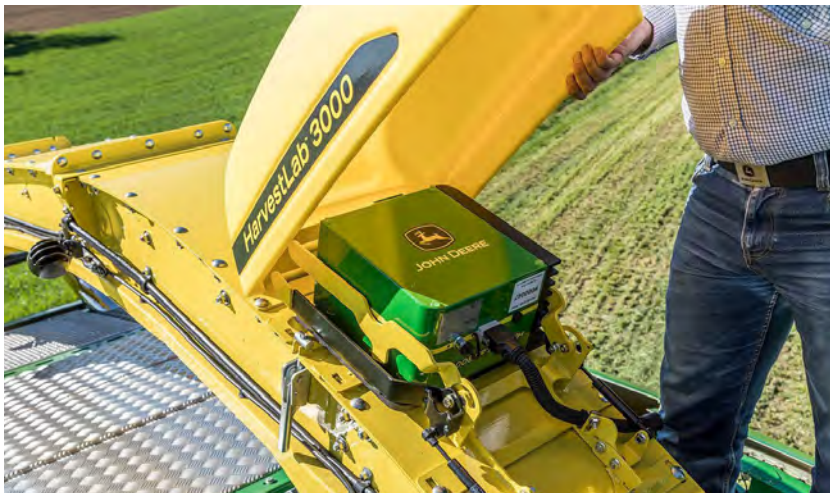
Onboard DM% scanning is become increasingly common (Image courtesy John Deere)
