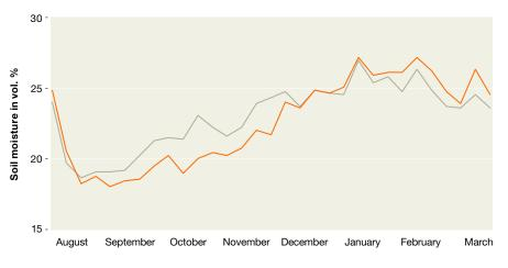
The DWD measured the effect of a freezing catch crop mixture compared to fallow on the soil water content from 0 - 60 cm over many years at the Threna site. The figure shows the course of the soil moisture content from August to March under the two variants. Compared to fallow, the catch crop has a more positive effect on soil moisture in spring and therefore does not have a negative effect on water availability in the following crop.
